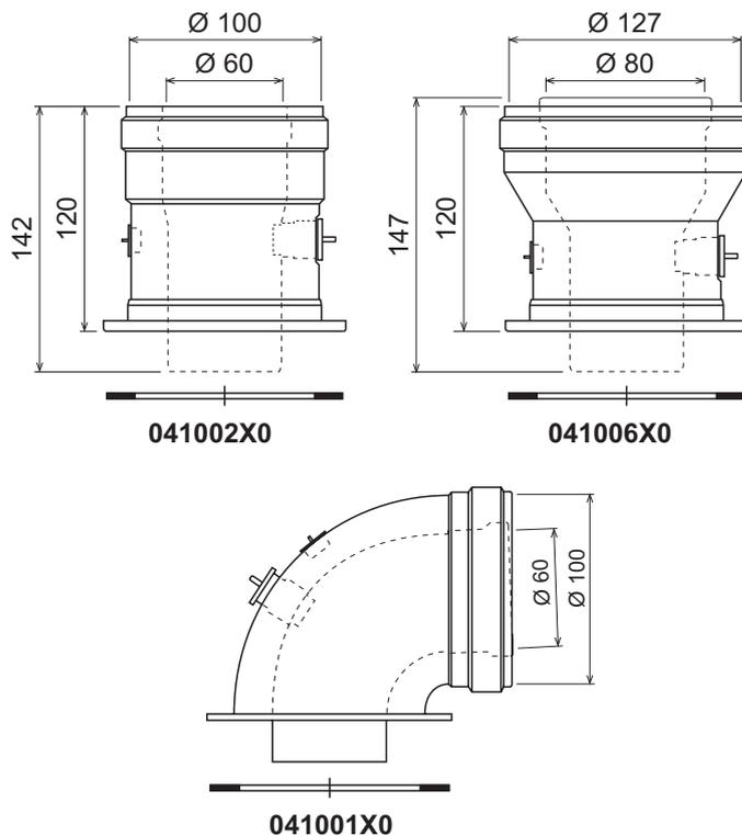
fig. 16 - Starting accessory for coaxial ducts
