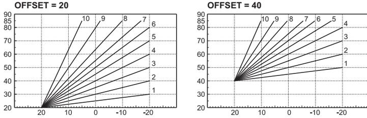
fig. 11 - Example of compensation parallel curve offset
