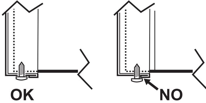
fig. 25 - Correct position of front panel
