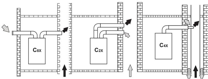
fig. 19 - Examples of connection to flues (⇨ = Air / ⇨ = Fumes)
