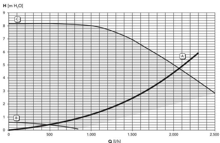
fig. 27 - Circulating pump head / pressure losses
