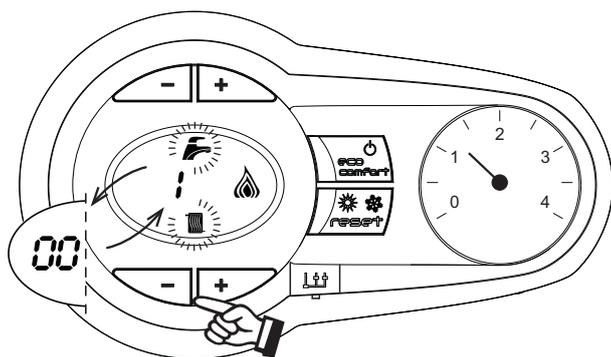
fig. 23 - Mode TEST (puissance chauffage = 100%)
