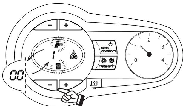
fig. 23 - TEST mode (heating power = 100%)
