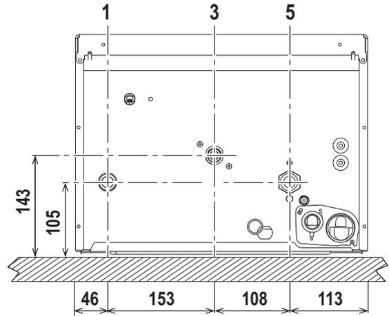
fig. 12 - Plumbing connections
